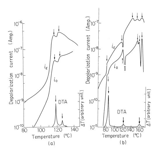
Fig. 2. TSC curves of smectic liquid crystals.
