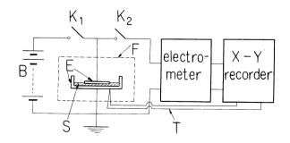
Fig. 1. A schematic diagram of the apparatus used for measuring the depolarization current.
